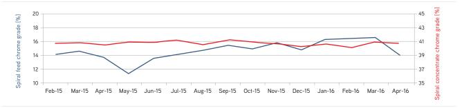
The results were achieved through manual adjustments on the cutter positions. Real-time indications from a MQi Slurry analyser installed on the product stream were used as a guide for these adjustments.
