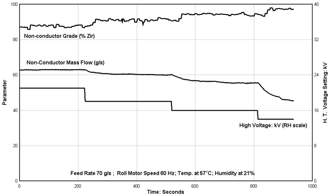
Figure 5: Impact of voltage settings on separator performance
