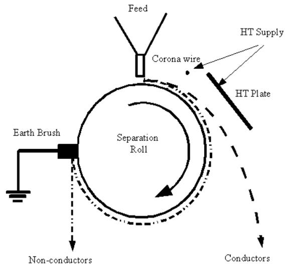
Figure 1: Schematic of a High Tension Roll Separator
