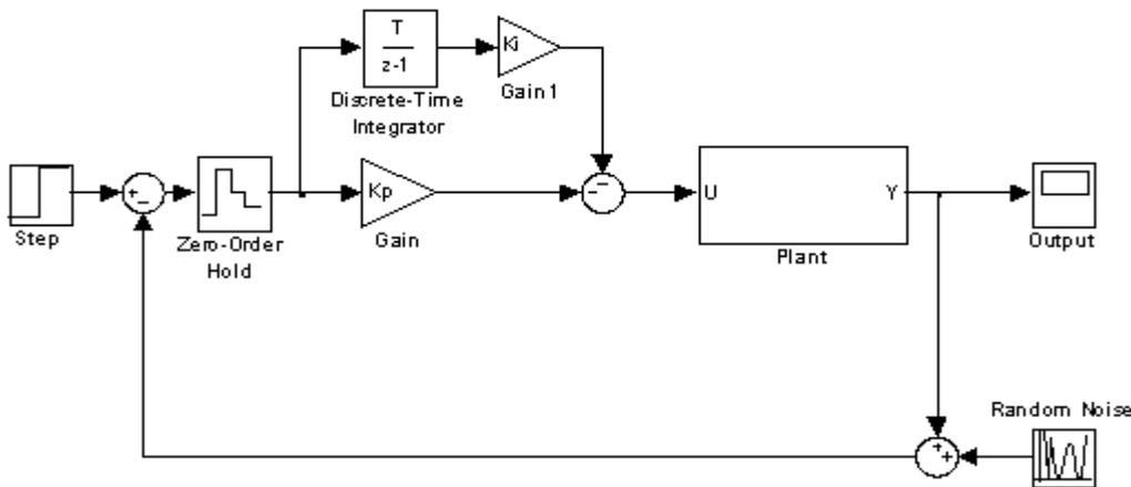
Figure 7: Control system for the pilot plant
