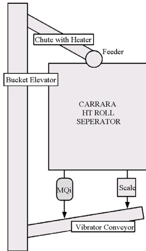
Figure 2: Schematic of Pilot Plant
